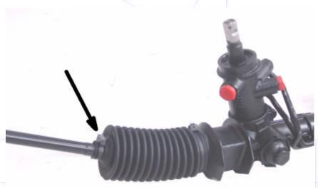
When mounting the tie rod ends and after the alignment of the wheels, the boots are not loosened.
